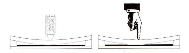
The MagnetoPot is a sealed potentiometer, in the membrane potentiometer tradition, yet it does not require a wiper/actuator to connect the collector and the resistor. Instead, the MagnetoPot is controlled by an outside magnet, which attracts the magnetic forces within the MagnetoPot to connect to the linear resistor and give linear potentiometer feedback.
